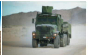
MTVR The Medium Tactical Vehicle Replacement carries up to 7 tons off-road. It’s an all-terrain workhorse with 21st century technologies.
