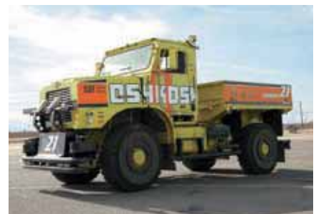
The remarkable TerraMax™ unmanned ground vehicle autonomously navigates a range of rugged landscapes. It earned a spot in the finals of the 2007 DARPA Urban Challenge.
