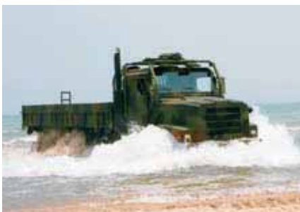
The Oshkosh® Medium Tactical Vehicle Replacement (MTVR) outruns, outlasts and outmaneuvers any other truck. It carries up to 7.1 tons off-road and 15 tons on-road.
