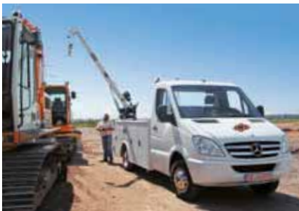
The IMT Dominator® field service vehicle is the first of its kind in the European market, with versatile service functions and integrated body, telescopic crane and air systems.
